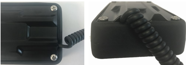
Figure 2. Sensor cable fed through slot
